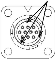
Plug connector key (Concavity)
