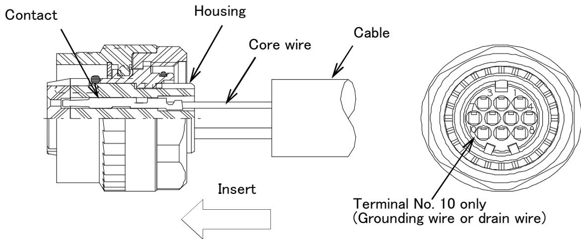
\* Insert the contact so that the lance and the terminal number face the same direction.
