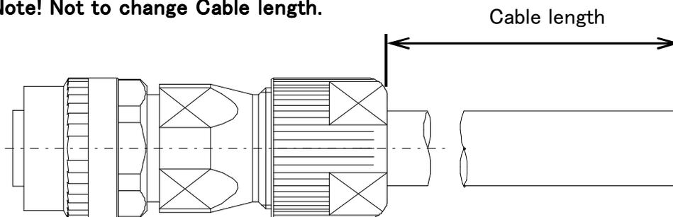
**\*Cable length after cutting =  $35 \pm 0.5$ mm for CM10-SPXXS(D6) + cable length
