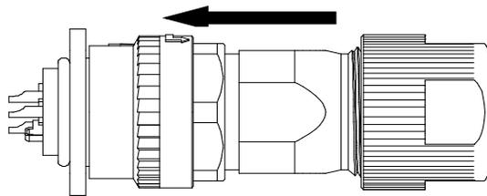
\*To remove, rotate the coupling and pull out to straight.
