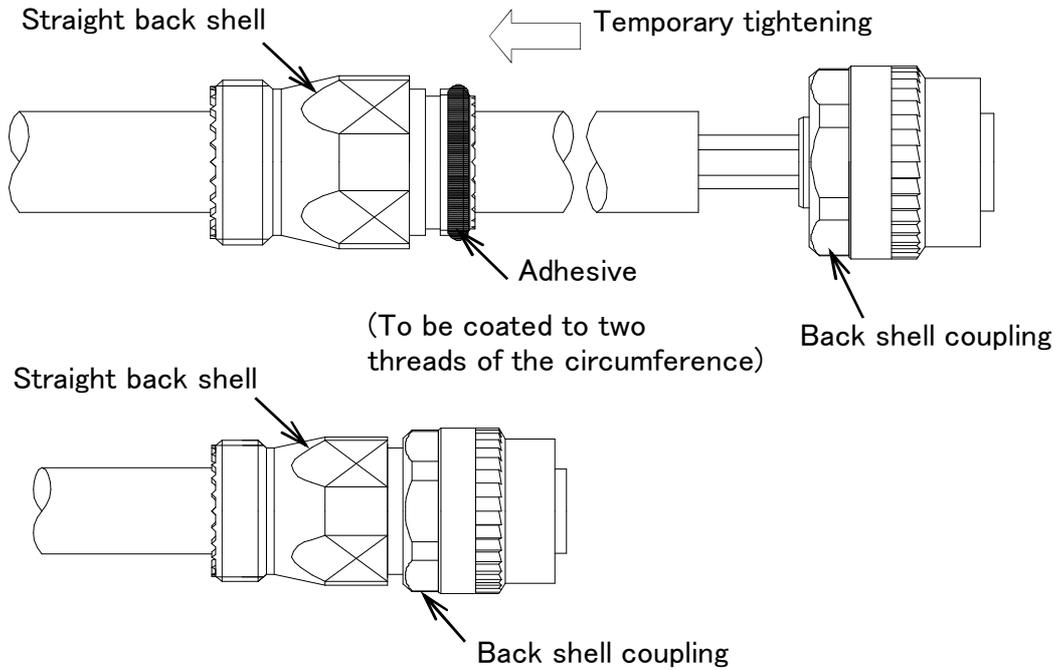
\* When tightening temporarily, match the concavity and convexity of the plug shell with those shell of the straight back shell.
